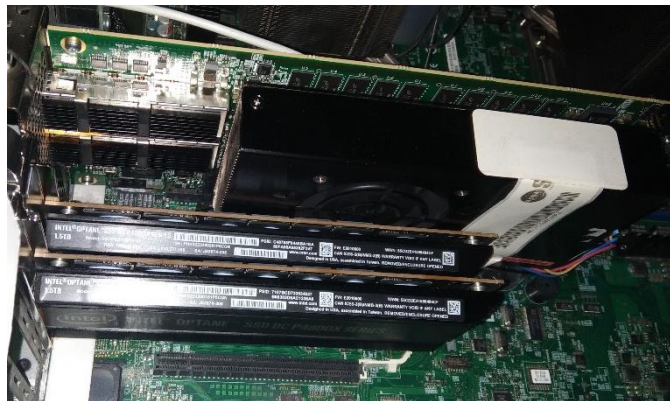
Figure 9: FPGA and SSD devices connected on the same server motherboard.
